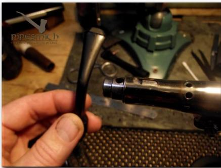
Before heating the stem for bending, you'll need to insert a pipe cleaner or similar to prevent collapsing or pinching of the stem's bore.
