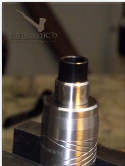
\*\*\*Using sand paper or a file, make sure to scuff the portion of the adapter that will be seated in the stem.\*\*\*
