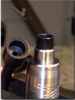
With the insert fully seated, clean both the outer surface of the insert and the inner chamber of the stem blank with alcohol.
