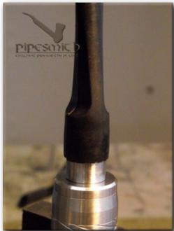
Using your choice of heat source, heat the base of the stem. Take your time and heat the base thoroughly and evenly, while taking care to not scorch or blister the stem surface.
