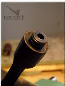
Once the adhesive has been allowed to completely cure, remove the stem from the atomizer using a twisting/ pulling motion (never rock a stem side-to-side to remove).
