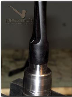
Test fit the stem blank to the atomizer that you will be using for setting up the stem. Any light adjustments to the base necessary to establish a solid and square seating should be taken care of now. Note: this refers to adjustments to the chamfered base only, and will apply primarily to seating the stem against an atomizer with a flat top. Adjustments to the stem diameter to achieve more fluid line of transition from atomizer to stem will be taken care of later.
